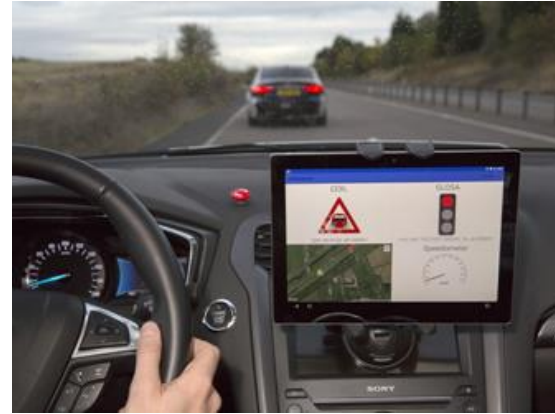
Electronic Emergency Brake Light (EEBL)
